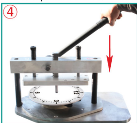
Place base ,mould B & A into machine table. Press the finished clock to punch a hole.
